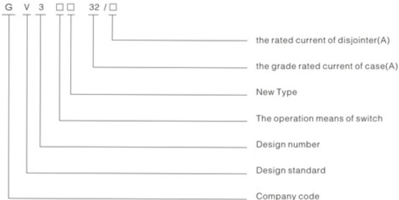
(GV2) Motor protection circuit breaker
