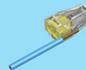
First Step strip the wire 10-12mm
