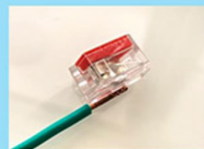
First Step strip the wire 10-12mm
